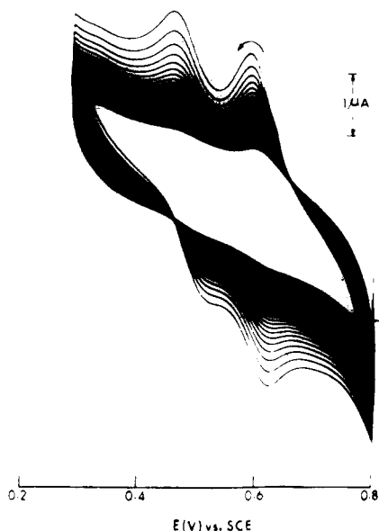
Figure 4. Repetitive scan cyclic voltammograms of incorporated \text{NiL}^{2+} at pH 8.35. Scan rate is 0.05 V/s, and total scanning time is approximately 30 min.
